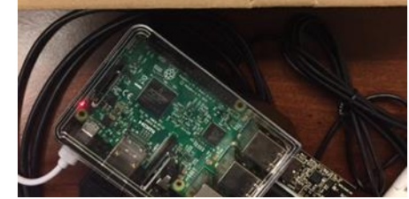
Portable mousejack attack kit
